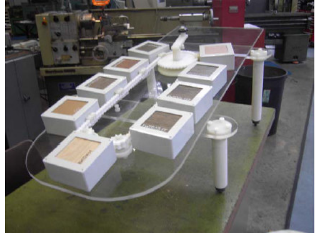
Figure 4. Photograph of the presentation apparatus used for tactile exploration experiments in the fMRI scanner.
