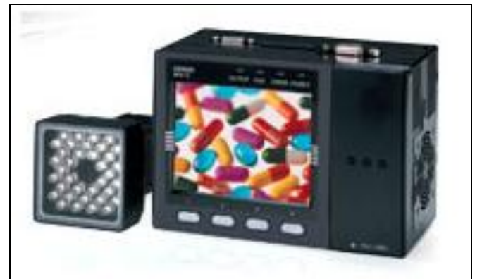
Fig. 02 The OMRON ZFX-C smart vision sensor system http://www.ia.omron.com/product/family/1892/index_fea.html
