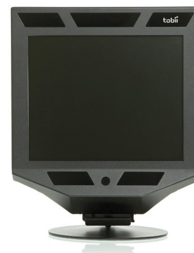
Fig.2. The Tobii 1750 eyetracker display with 2 infrared diode trackers and central camera at the bottom of the screen.
