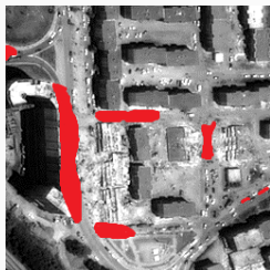
Figure 11: (b) Road damage detection
