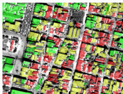
Figure 2: Damage detection and assessment
